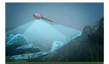
HUGIN is an underwater vehicle that is used for highresolution mapping of the sea floor, pipeline inspection and detection of gas leaks from shallow water to the ocean depths. The technology contributes to the sustainable management of the sea, security, energy production, marine research and not least widening our knowledge and understanding which is necessary for the beneficial co-existence between nature and aquaculture.
