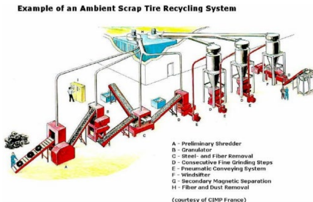
Figure V Schematic of an ambient waste tyre processing plant
